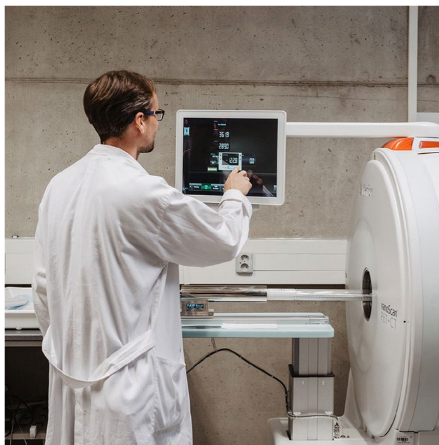
◀ EATRIS – Evaluation of pharmacokinetics and distribution of candidate radiopharmaceutical in experimental animals using positron emission and computer tomography
